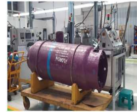
Station-1 AFTER Solution Implemented: To eliminate the productivity loss caused by this process, a separate hydraulically operated chain hoist was made with available raw material generated through unused inventory. With simple Push button operator can load this e drive on Cradle fixture precisely without losing balance. 1. Solution was conceived within the company, no external help was required. 2. HIRA was reviewed to tackle and manage these changes. 3. Cycle time improvement of 60 sec 4. 1 Man Saving for the operation
