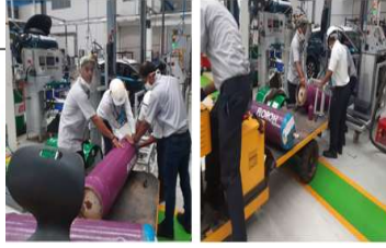
Station-1 BEFORE Description of Activity being performed: E drive consisting of induction motor & gear box required to be mounted on cradle assembly for assembly activity. This lifting of e drive from pallet is being done with Belt & crane 1. As belt has to be put in lifting tackles on e drive, there becomes unbalance in the load causing wobbling movement of e drive which was resulting in inaccurate positioning of e drive on fixture causing fall hazard. 2. Ergonomically it is not recommended process as heavy load gets on the hand while doing the adjustment to mount e drive on fixture. This was time consuming activity and usually 2 Men are required to perform the task.
