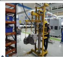
Station-1 AFTER Solution Implemented: To eliminate the productivity loss caused by this process, a separate hydraulically operated chain hoist was made with available raw material generated through unused inventory. With simple Push button operator can load this e drive on Cradle fixture precisely without losing balance. 1. Solution was conceived within the company, no external help was required. 2. HIRA was reviewed to tackle and manage these changes. 3. Cycle time improvement of 60 sec 4. 1 Man Saving for the operation
